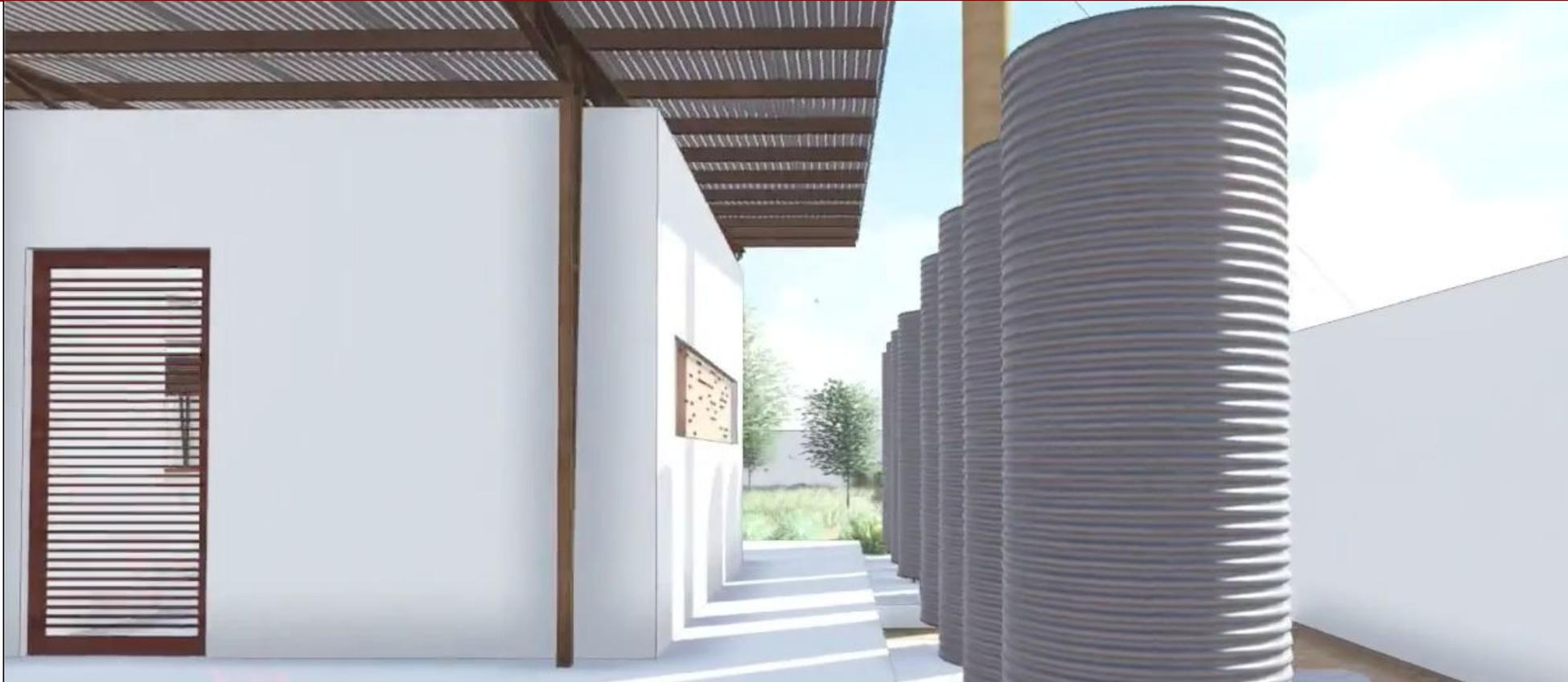
The center has an installation system that stores rainwater in reservoirs to reuse it in watering the garden. A way to reduce the consumption of tap water.
