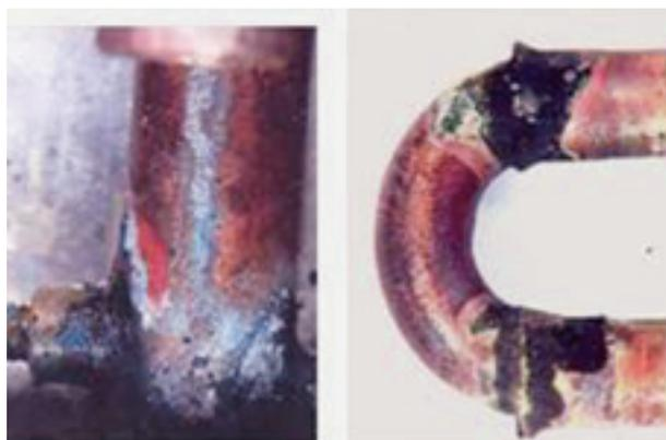
Picture 13: Corrosion on the hot copper tubes and the silver-containing brazed joints.
